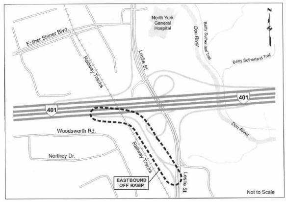
The Ministry of Transportation (MTO) is undertaking the re-alignment of the eastbound off-ramp at the Highway 401 and Leslie Street Interchange. As part of the re-alignment, construction activities will also include replacement of the Metrolinx pedestrian bridge; upgrading of traffic signals at the W-N/S ramp terminal intersection; and replacement of the noise barrier where impacted by construction.
